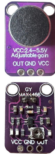
Figure 4.1: Electret Microphone with Amplifier Circuit
