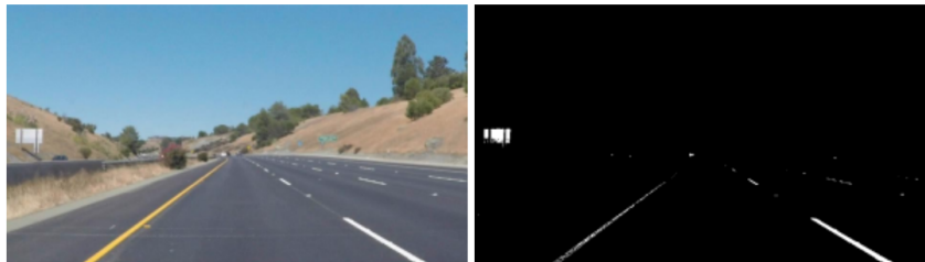
Fig. 3.4 Before (left) and after (right) the application of the threshold, test image
