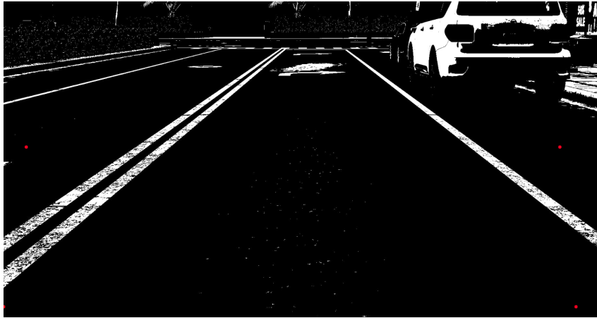
Fig. 3.5 Threshold applied in the CARLA simulation environment
