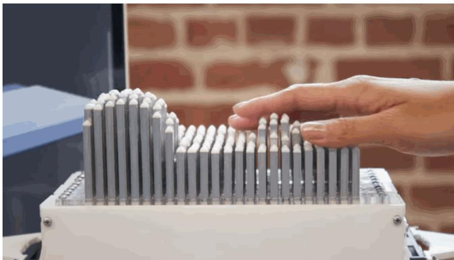
**Figure 6.2:** Tactile display by Stanford University
