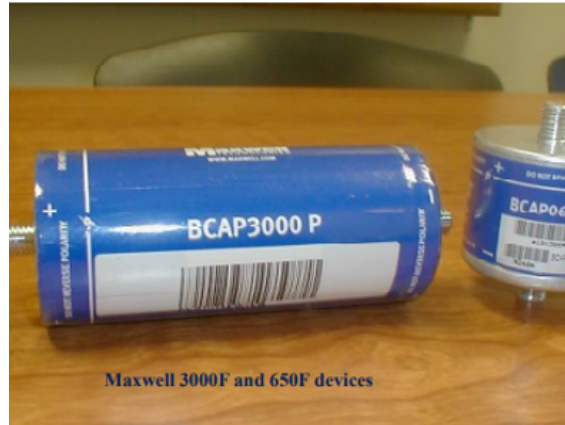
Figure 2.5: Maxwell 3000F SUPE
