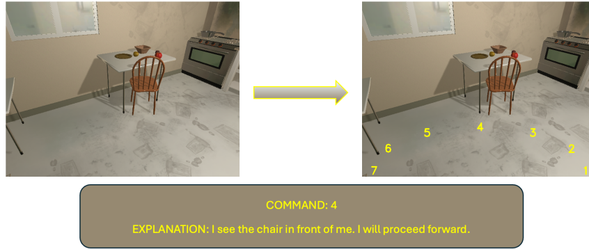
Figure 3.6: Visualization of the decision-making process by the robot. The left image shows the initial scene with the chair in front of the robot. The right image highlights the robot’s forward movement based on the command issued (Command: 4), as indicated by the numbered path markers. The explanation box describes the robot’s reasoning: "I see the chair in front of me. I will proceed forward," demonstrating how visual inputs and navigation decisions are processed.
