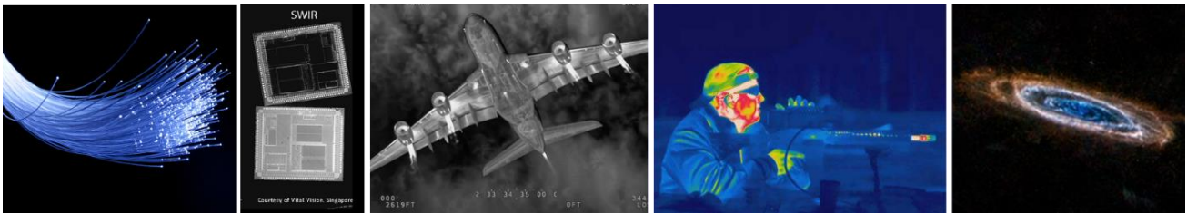
Figure 1: typical applications of the different regions of the infrared spectrum. From left to right: NIR is the typical wavelength for telecommunication, due to the low absorption of optic fibers in this range. SWIR image of a silicon chip, which due to its transparency in this region allows for easy detection of defects. MWIR of a plane, with a strong signal emitted from the high-temperature exhaust gasses. LWIR image of a soldier holding a rifle. FIR image of the Andromeda galaxy from the Herschel Space Observatory.
