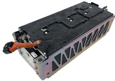
(b) Module of Honda Clarity [53].
