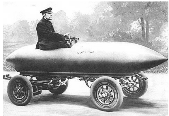
(b) The Camille Jenatzy speed record Jamais Contente electric vehicle (1898) [45].
