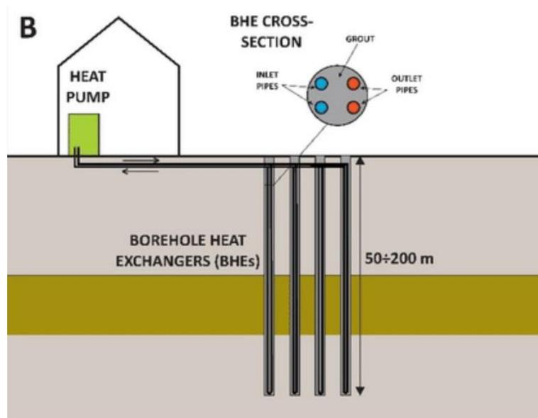
*Figure 6 representation of a vertical closed loop system*
