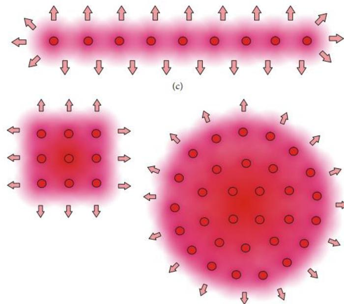
Figure 37 Different array shapes for BTES
