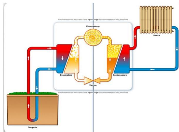
Figure 9 Operating scheme of an heat pump
