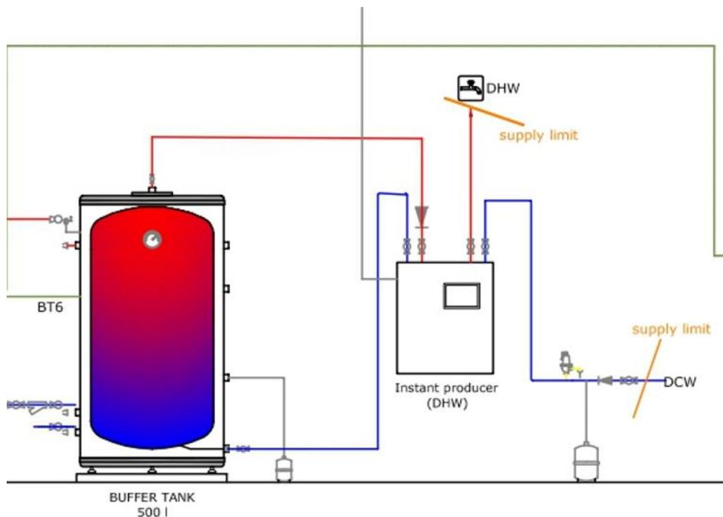
Figure 34 Buffer tank and instant producer, Geonovis 2024
