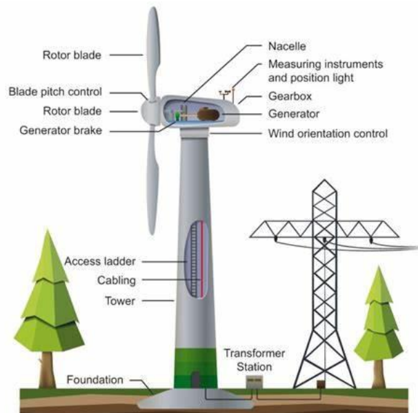
Figure 37 - Main components of a wind turbine [32]
