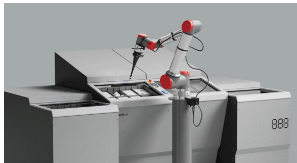
Figure 18 Cobot installed on Autostore, Source: [14]
