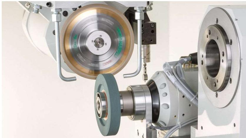
Figure 14. Cross-axis dressing configuration (5).
