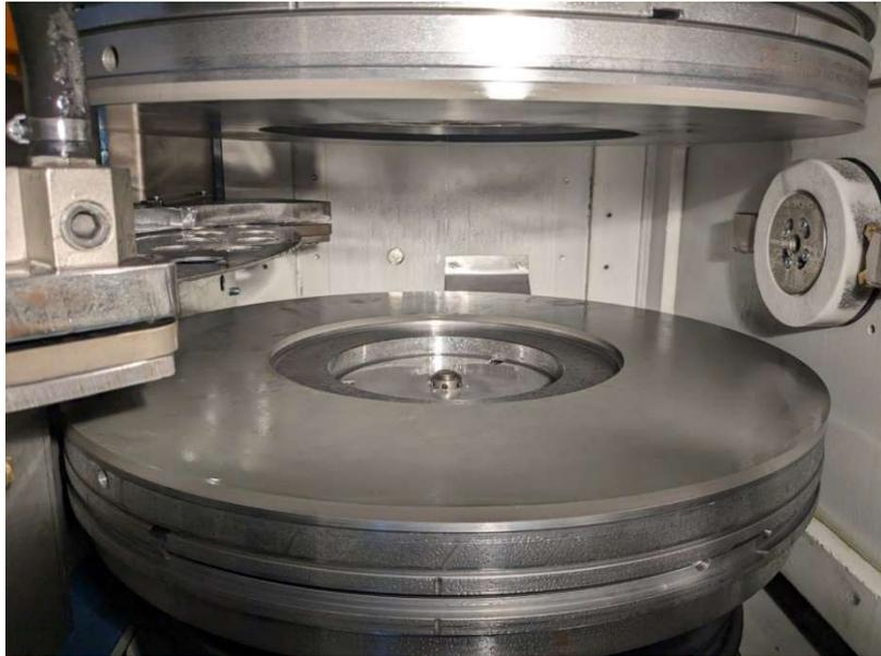
Figure 17. Top and bottom grinding wheels
