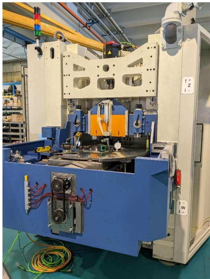
Figure 16. Monzesi Viotto vertical spindle double disc grinding machine.
