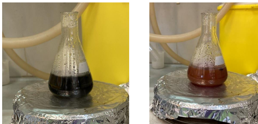
Figure 5: Steps in the procedure of synthesizing spherical gold nanoparticles of 70nm in diameter. Color change after a given timing.
