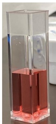
Figure 33 : The wide-path cuvette with 1 ml of colloidal solution of spherical Nps for UV-Vis analysis.
