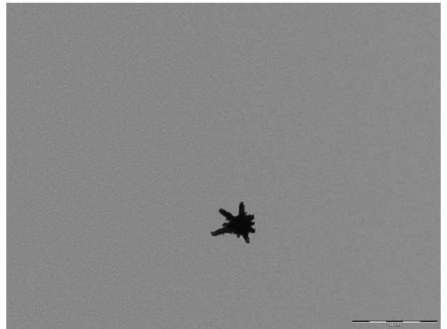
Figure31: Star-Shape nanoparticles of 19nm seen by TEM microscopy at 500nm magnification
