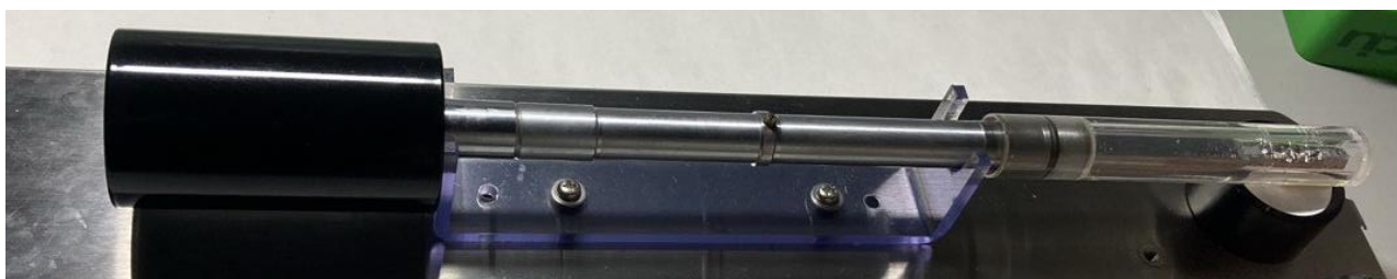
Figure 6: In the red circle is where the samples are inserted. Two TEM grids can be inserted at a time and then analyzed individually one after the other.
