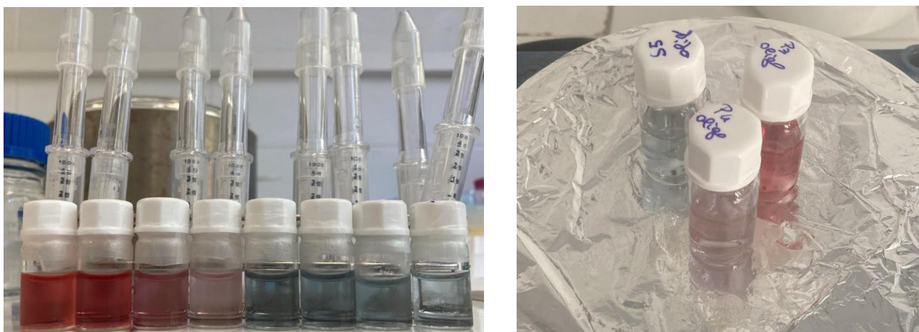
Figure 16: A) the synthesized nanoparticles and the nanoparticles with the oligo. B) Nanoparticles during functionalization steps on the stirrer.
