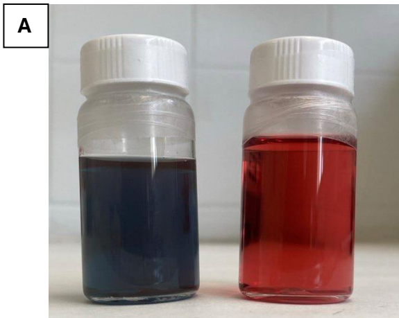
Figure 15 A :Gold nanoparticles in colloidal solution: in red the spherical nanoparticles(10-20nm) and in blue the star-shaped nanoparticles (>70 nm).
