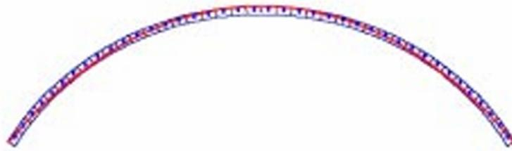
Figure 2.12. A Bare arch, where the red line shows the line of thrust [16].
