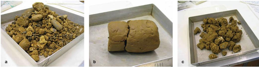
Figure 2.6. Backfill materials taken from bridge trial pits: a) granular, b) cohesive, c) other (cohesive-frictional) [12].
