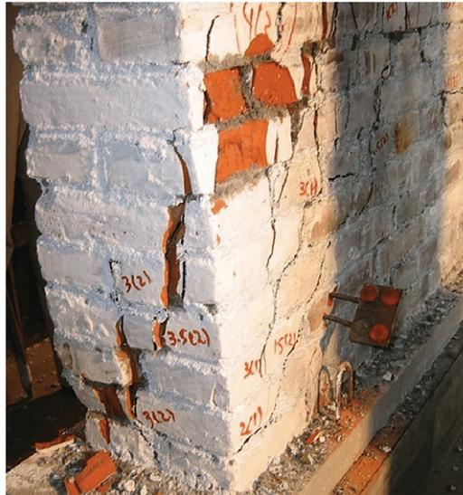
Figure 2.4. Brickwork test specimen under high pre-compression showing failure due to formation of tensile cracks [12].
