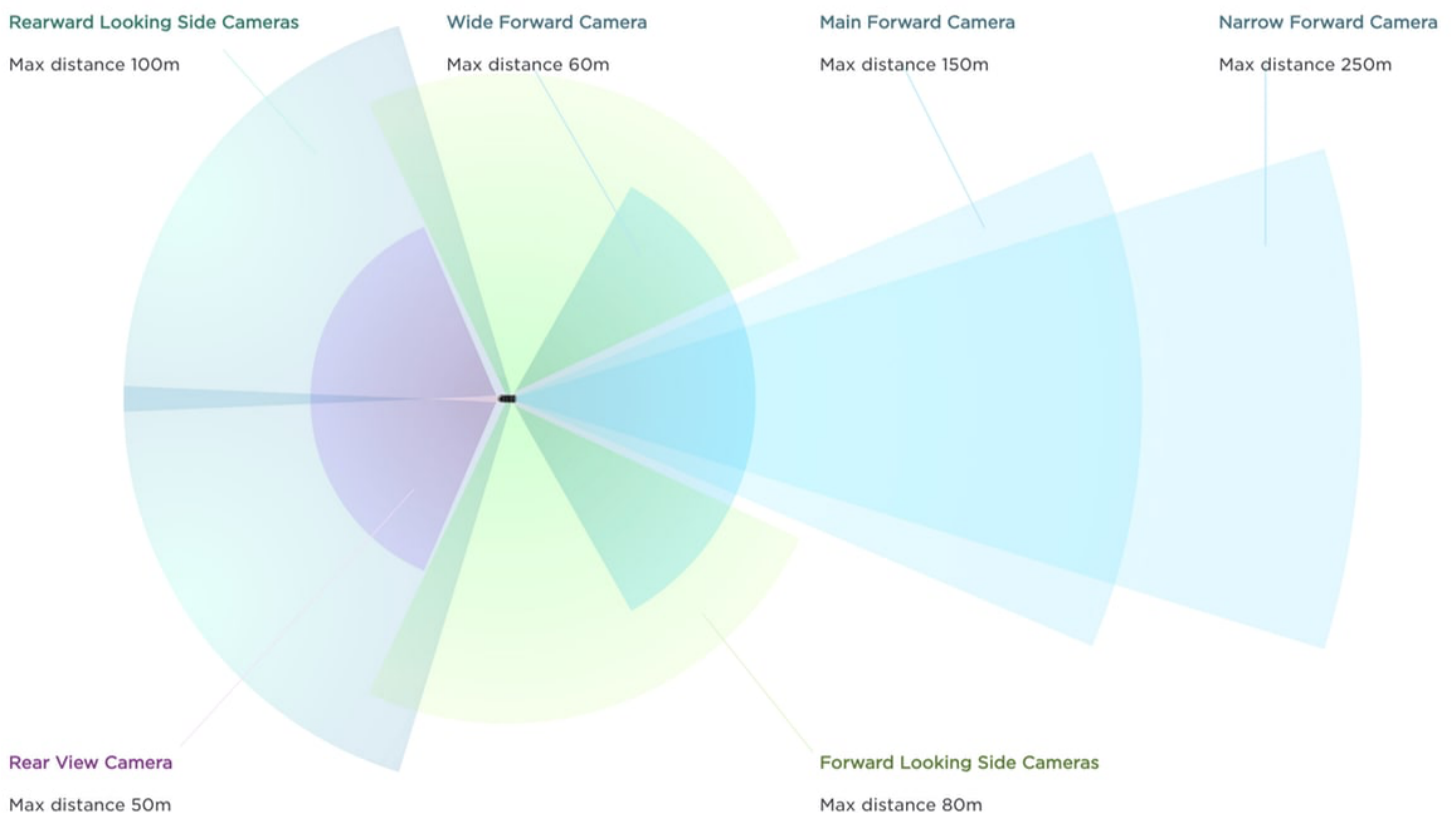
Figure 7: Tesla's camera around placed strategically around the vehicle
