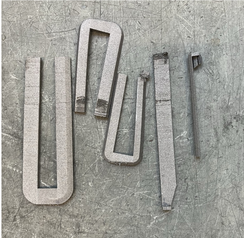
Figure 3.5: Result of the AlSi10Mg print part 2.
