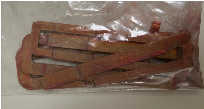
Figure 3.3: Winding printed in copper after shot peening.
