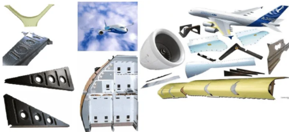
Figure 1.3: Aircraft components that incorporate composite materials [11].
