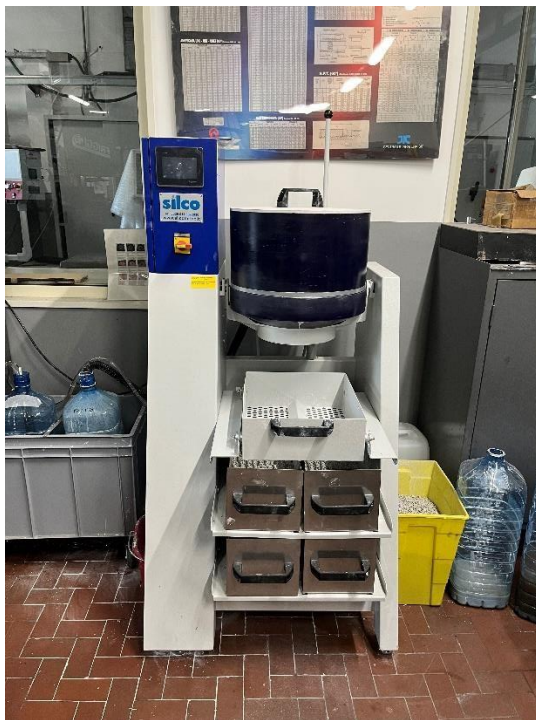
Fig. 45: The equipment from Silco employed to carry out tumble-finishing on specimens in their as-built state.
