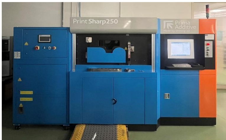
Fig. 44: The industrial machine utilized is the Print Sharp 250 by Prima Additive in L-PBF.
