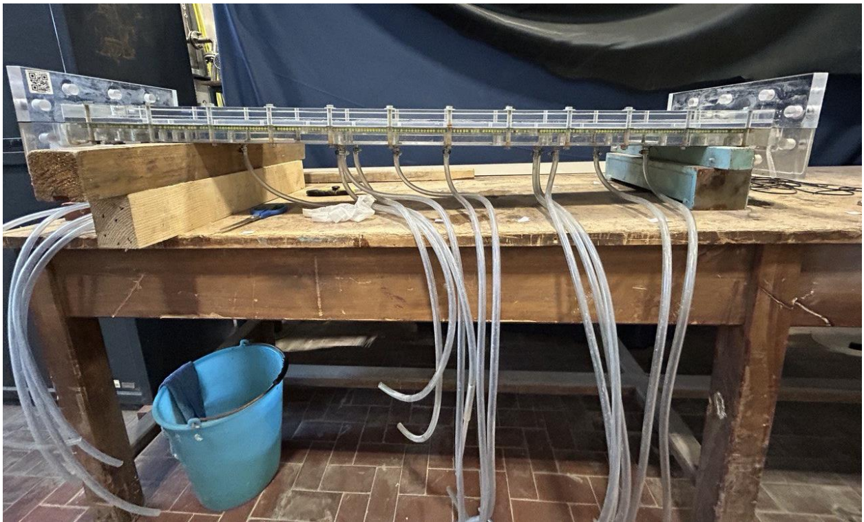
Fig.15 Drainage Tube System.
