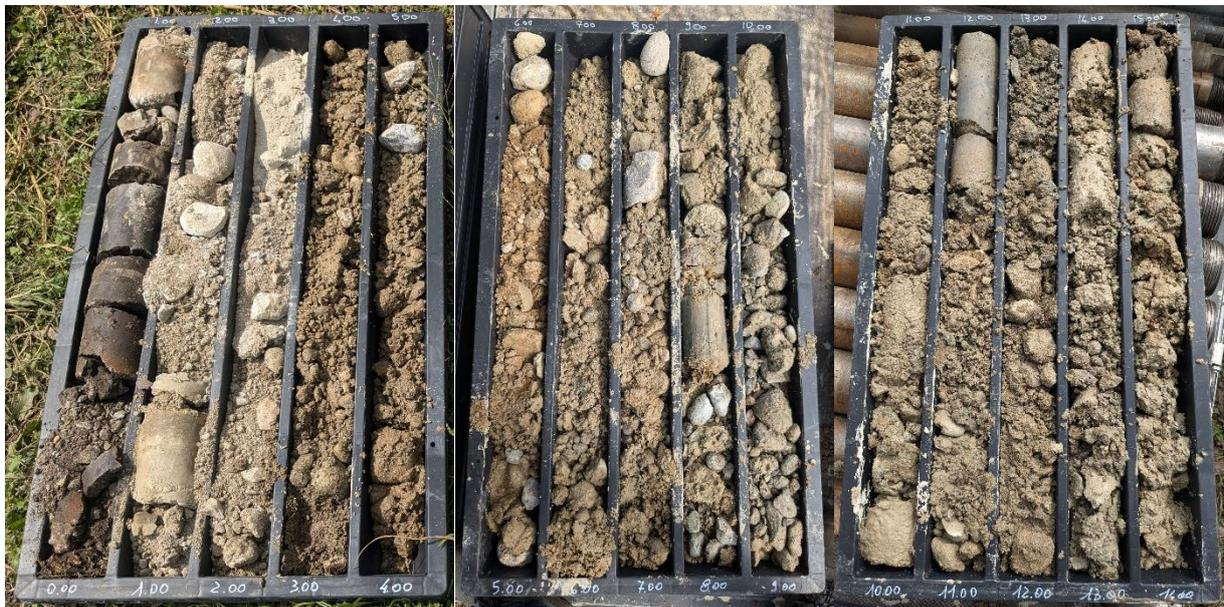
Figure 90. Cores retrieved from the drilling bit during the excavation of the new monitoring well. Every box contains 5 m of cores.
