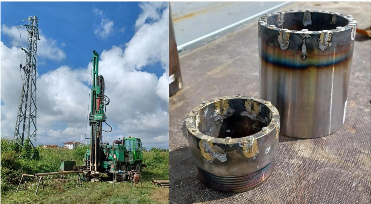
Figure 88. Drilling machine (left) and drilling bits (right) for the excavation of a new monitoring well in Trucchi (CN).
