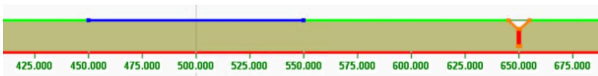
Figure 79. MAR 2D and Fontanile - Zoom on the Geometry and B.C.: no flux (red), atmospheric (green), variable flux (blue), seepage face (orange). The furrow is located at 100 m from the end of the injection trench.
