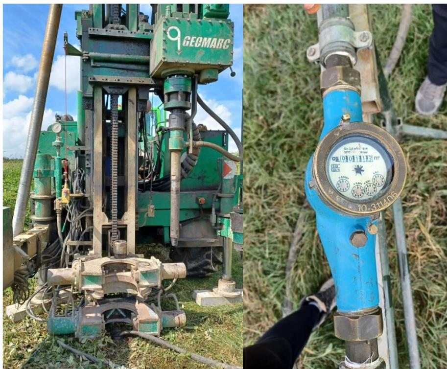
Figure 89. LeFranc Test: the pipe at the top of the excavation ready to inject the water (left) and the water meter for the measurement of  $Q$  (right).
