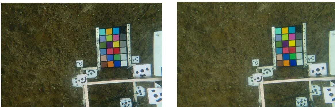
Figure 111 - Comparison of original image (left) and radiometric correction with ColourChecker (right)
