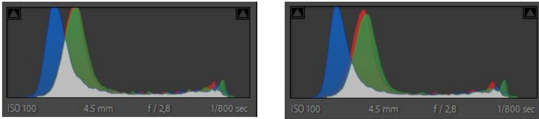
*Figure 112 - Comparison of original histogram (left) and radiometric correction with ColourChecker (right)*
