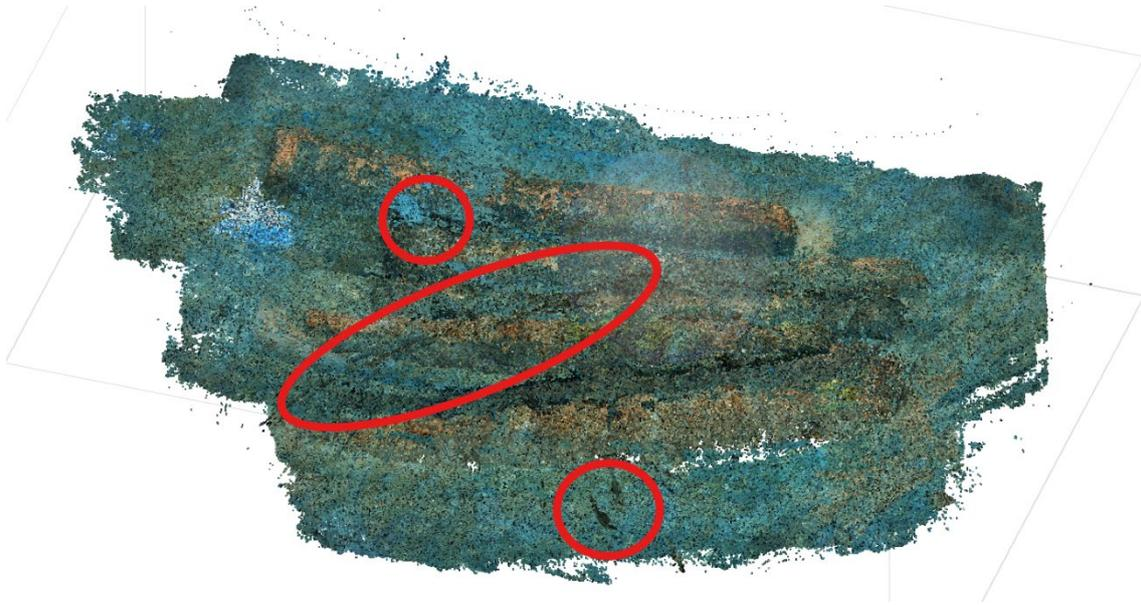
*Figure 118 - Point cloud with noise and misalignments*
