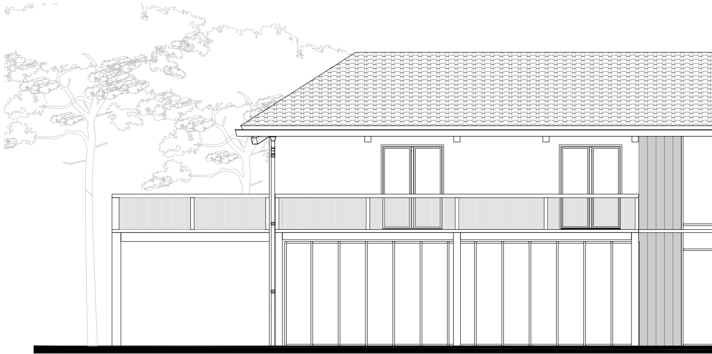
Figure 118. OPTIMIZATION SOUTH ELEVATION SCALE: 1/100
