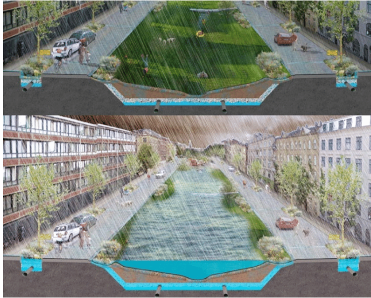
Figure 2.5: SuDS Features in Copenhagen
