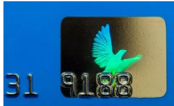
Figura 14_ brevetto Polaroid ologramma arcobaleno, (Jonathan Ross, Hologram Collection, http://www.jrholocollection.com/collection/benton.html )
