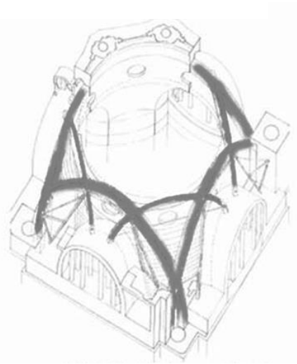
FIGURE 48- THE HIDDEN STRUCTURE IN 3D FORMAT FROM A RESEARCH PAPER "UNFOLDING SAN LORENZO" BY NTOVROS VASILEIOS
