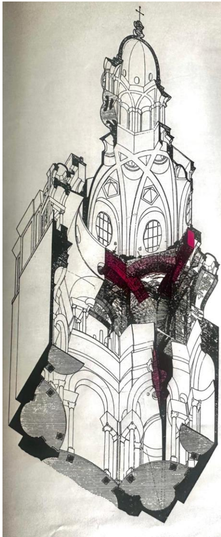
FIGURE 50- TURIN, S. LORENZO. AXONOMETRIC VIEW DEMONSTRATES THE HIDDEN STRUCTURE FROM 1920
