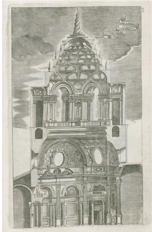
FIGURE 7- GUARINO GUARINI – ARCHITETTURA CIVILE – SECTION OF THE CHAPEL OF THE SHROUD (S. SINDONE)
