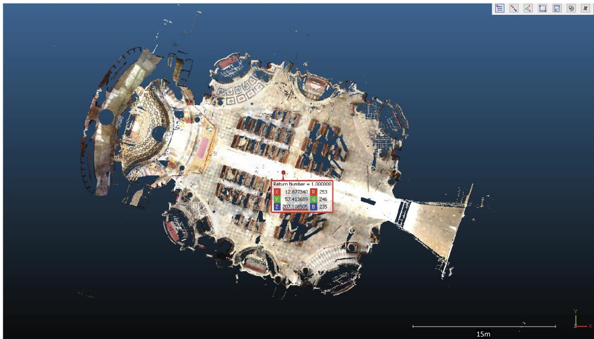
FIGURE 100- THE GROUND FLOOR POINT CLOUD PLAN AND THE COORDINATES OF A POINT ON THE FLAT SURFACE OF THE GROUND FLOOR ARE UTILIZED TO ACQUIRE THE RELATIVE HEIGHT QUANTITY WITH RESPECT TO THESE SPECIFIC COORDINATES. THE COORDINATE OF Z IS 207.11 METERS.
