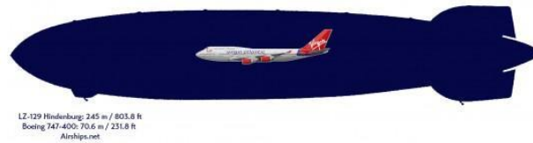
Figure 6: Size comparison between Hindenburg LZ-129 and Boeing 747-400 (airship.net).
