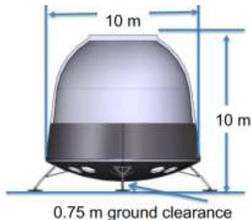
Figure 41: Capsule bottom and side with dimensions
