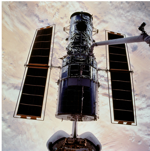
(b) Columbia's robotic arm dock Hubble in the shuttle's cargo bay (SM3B) [3]
