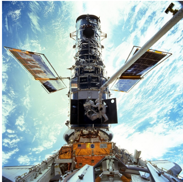
(a) Astronauts Steven L. Smith and John M. Grunsfeld replace Hubble's rate sensor units (SM3A) [3]
