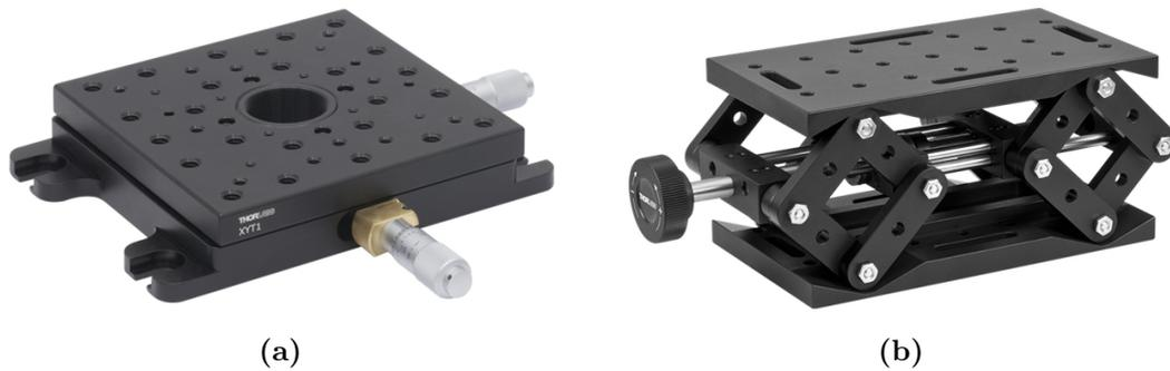
**Figura 3.28:** (a) Movimentatore lineare THORLABS®. (b) Lab Jack THORLABS®
