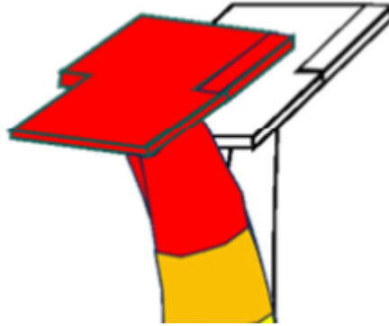
Figure 41: 1st Family Modeshapes - FLAP - TIGHT CONFIGURATION
