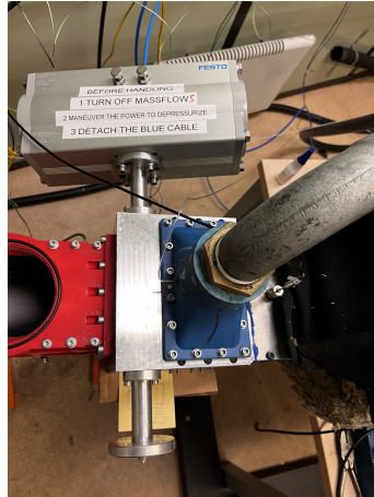
Figure 3.17: Three way valve
