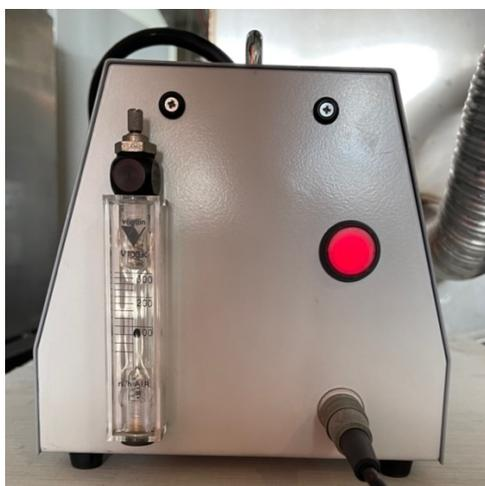
Figure 58 Flow meter for regulating aerosol output (TSI 3079A)
