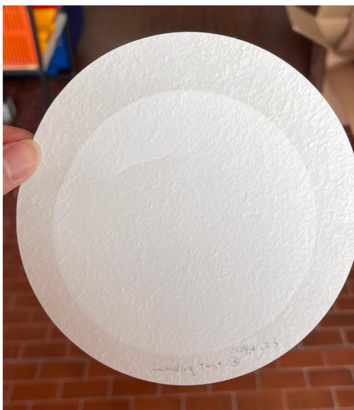
Figure 92 Loaded standard flat sheet media
