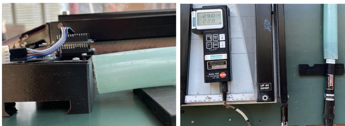
Figure 33 Measurement configurations: Left Nova fitness SDS011 with MKR ENV shield, Right RIP 02/02 temperature and RH probe inside tube
