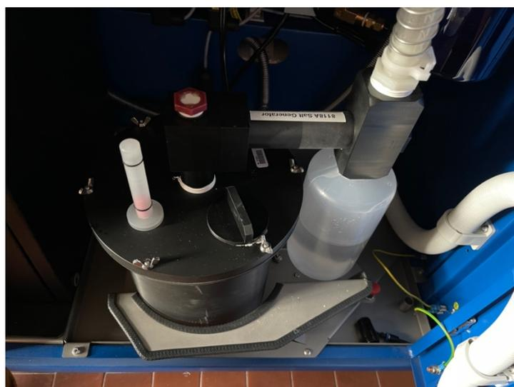
Figure 30 Aerosol generator NIOSH 8118A
