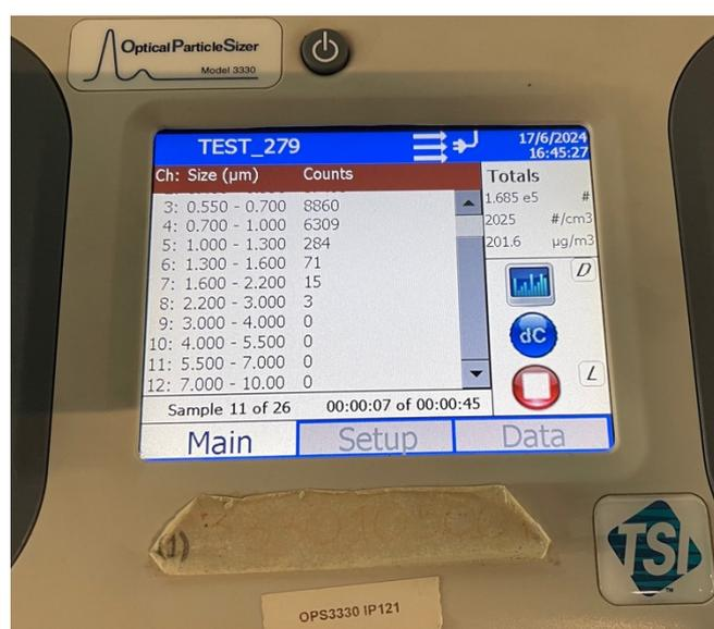
Figure 63 Particles detected by OPS3330 after activating the EAN 581
