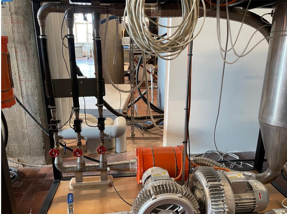
Figure 14 Mechanical valves for air flow adjustment and upstream and downstream fans
