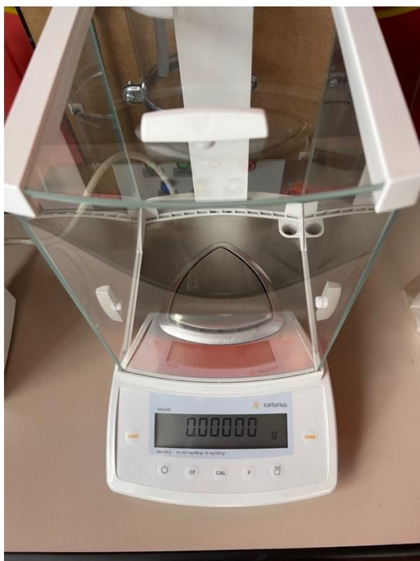
Figure 42 Sartorius balance with its precision
