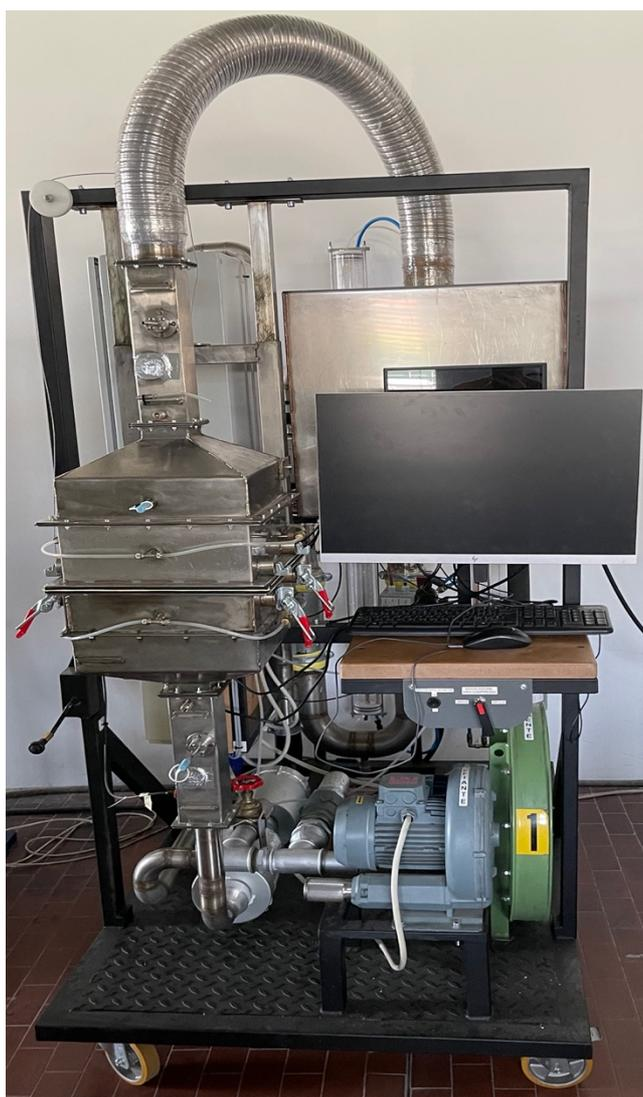
Figure 50 Test rig for RH control
