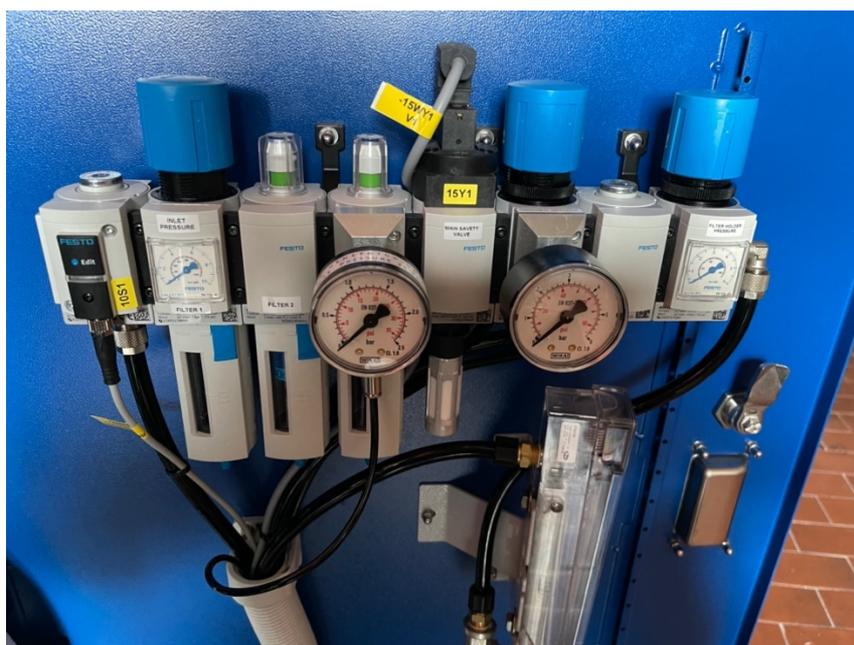
Figure 32 Valves for adjust pressure and flowrate
