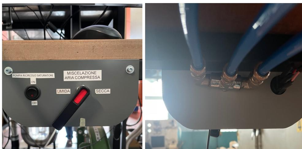
Figure 53 Handlebar for regulating opening of three-way valve for RH control (left) three-way
