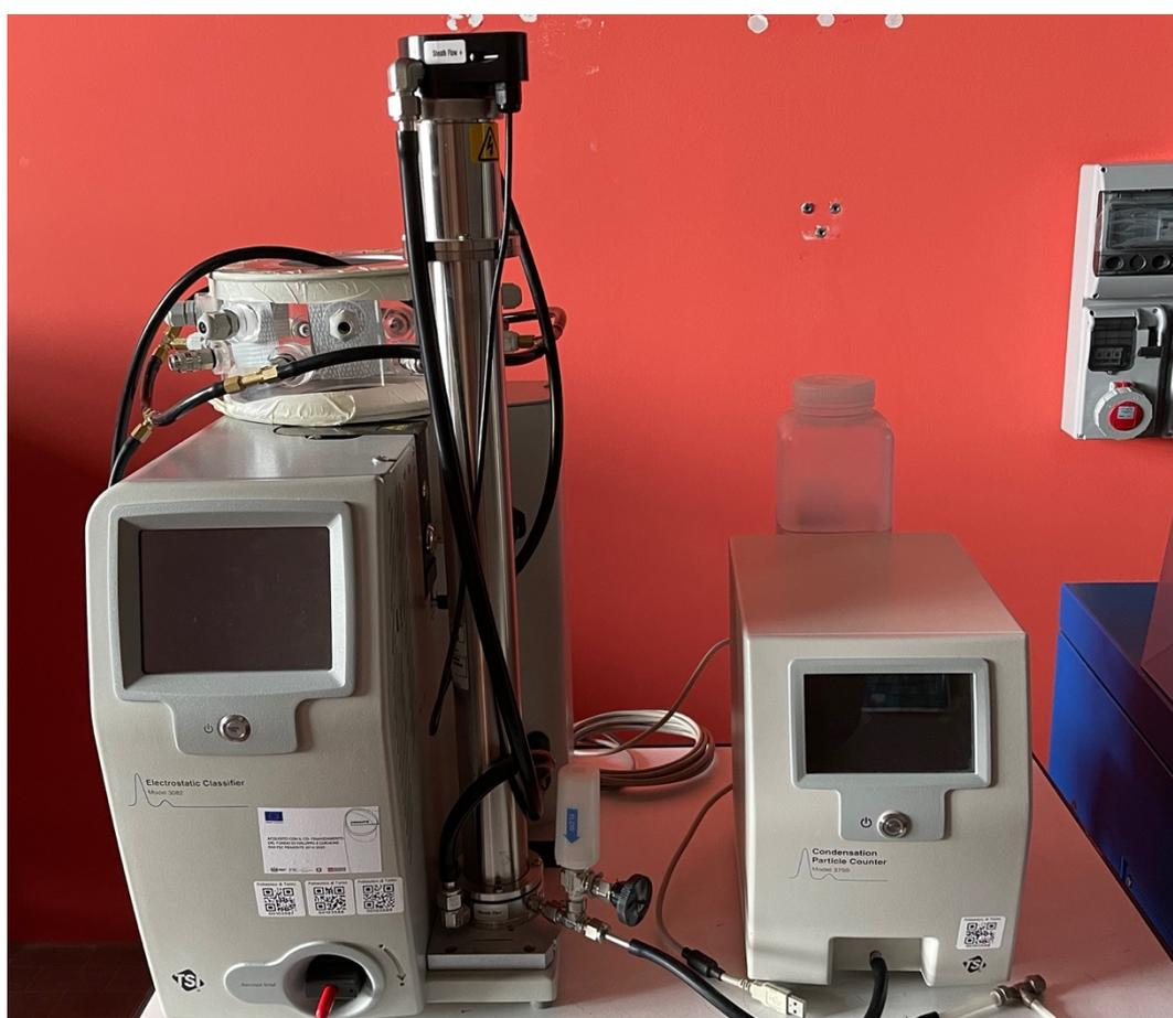
Figure 4 SMPS model 3938 consists of DMA and CPC for detecting electrical mobility of particles from 10nm to 1000nm
