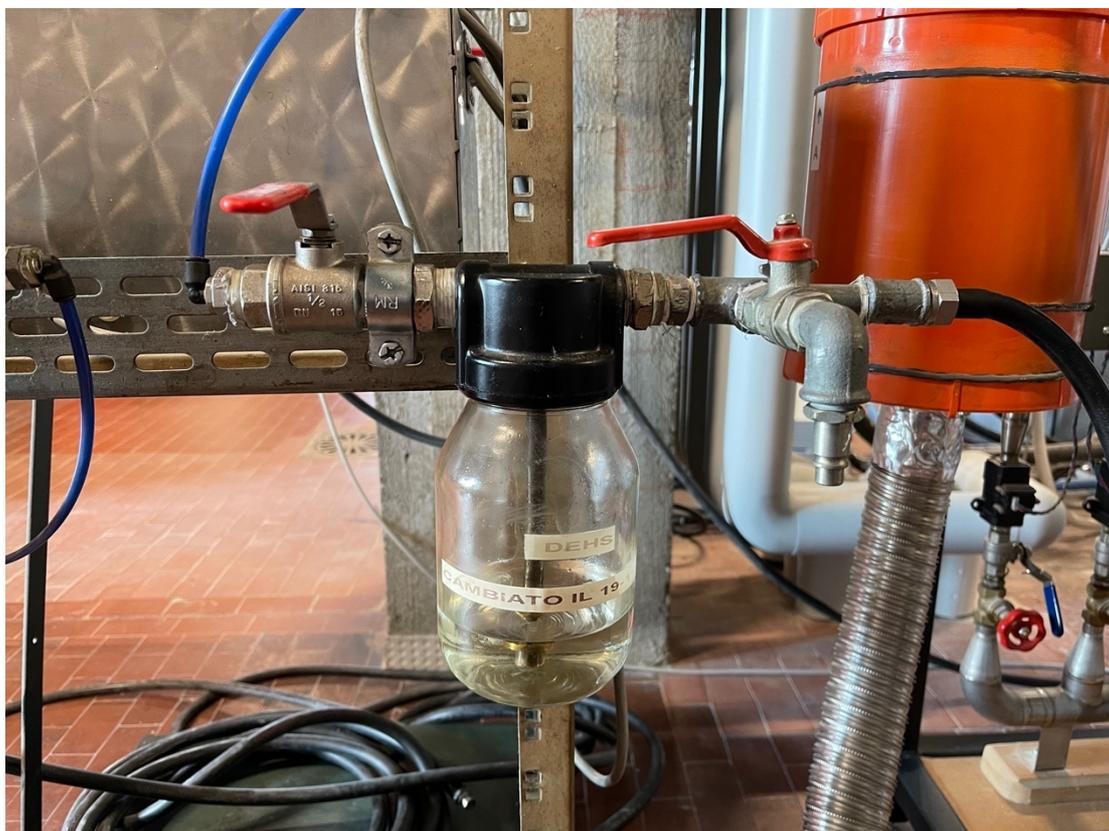
Figure 26 Liquid aerosol DEHS (DiEthylHexylSebacate) generator
