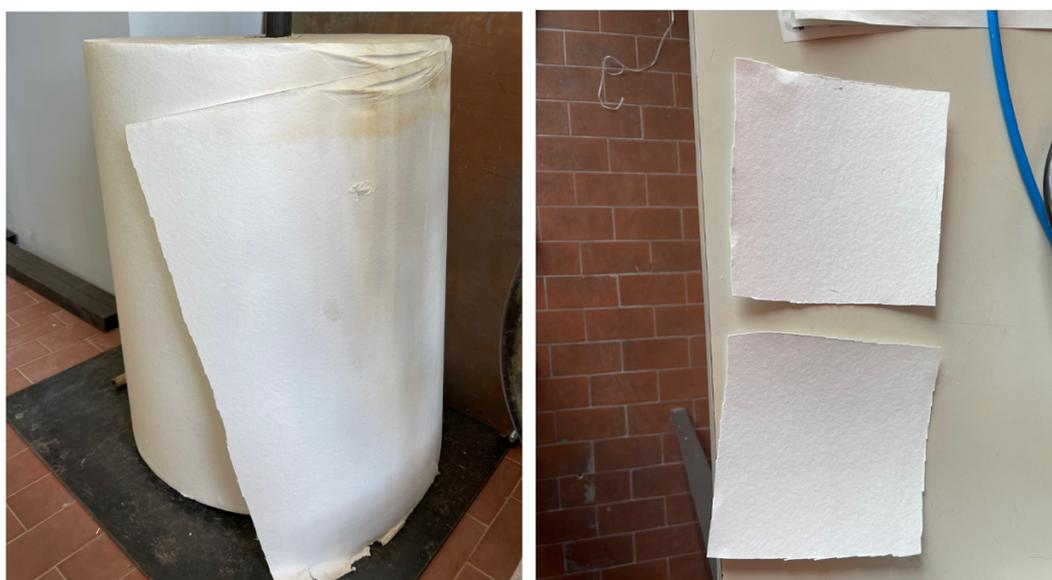
Figure 41 Second filter media: Left roll of filter media Right pieces of media cut from roll
