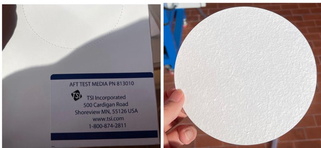
Figure 40 First filter media: Left package with information of media type Right clean media
