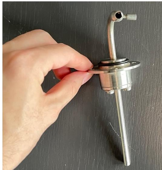
Figure 57 9mm aerosol sampling nozzle
