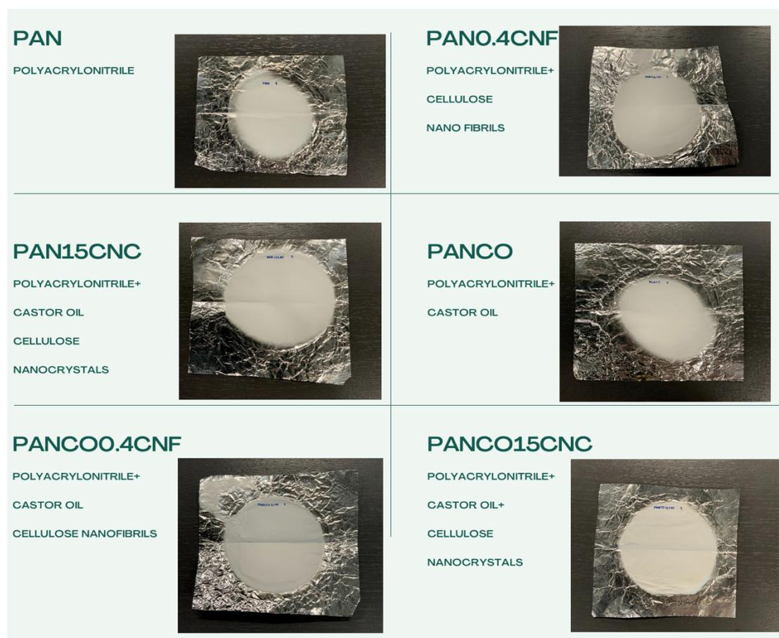
Figure 6 Test samples of nanofiber flat sheet media and their composition
