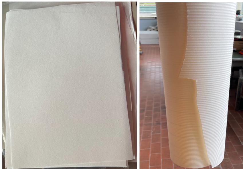
Figure 64 Left) Ahlstrom media for loading test Right) Technostat FA6900NW electrostatic media for tuning neutralizer
