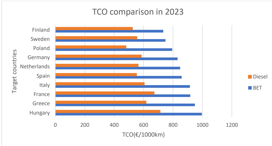
Figure 10 TCO comparison of diesel and BET trucks in 2023.
