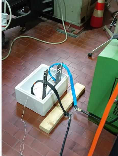
**Figure 4.26:** Superconducting tape setup surrounded by liquid nitrogen and insulator
