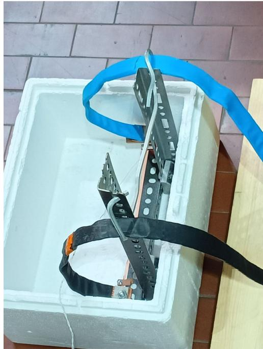
**Figure 4.25:** Superconducting tape setup surrounded by liquid nitrogen and insulator
