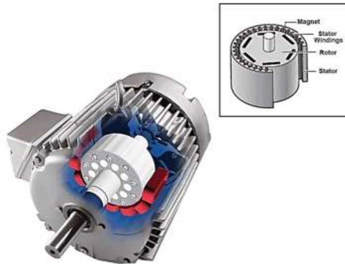
Figure3. PMSM Model Illustration, taken from [39]
