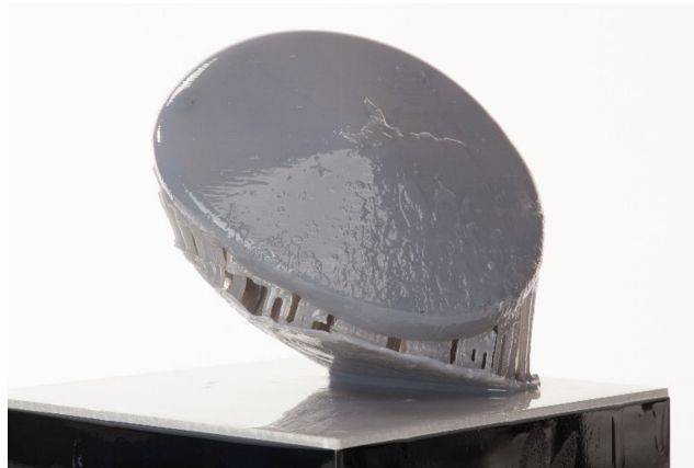
Figure 10: No adhesion on the building platform
