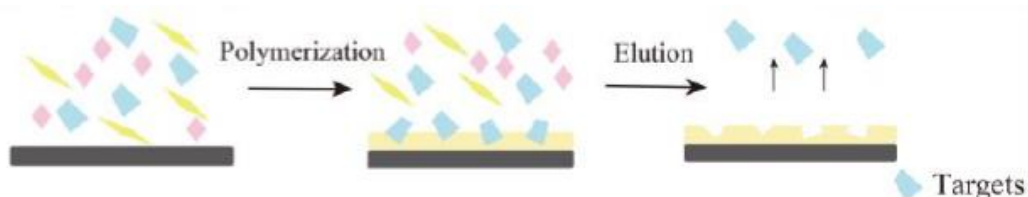
Fig. 10 Schematic Illustration of MIP synthesis by surface imprinting.[27]
