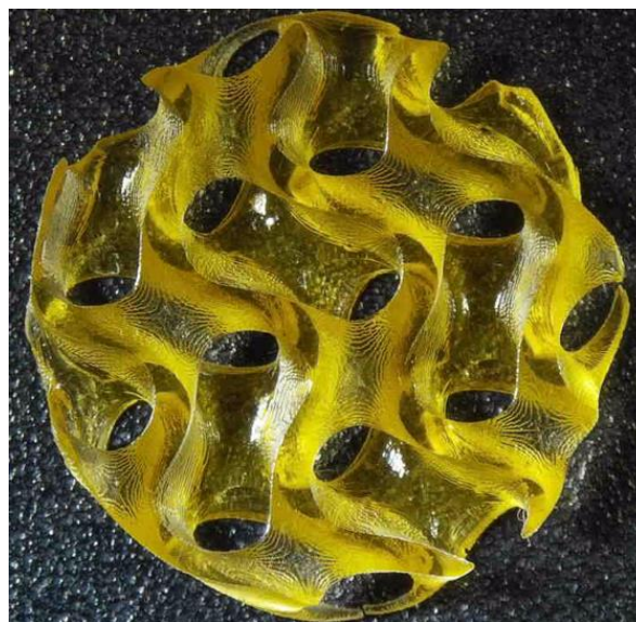
Fig. 32 Top view of a printed MIP gyroid. Image obtained with an optical microscope.
