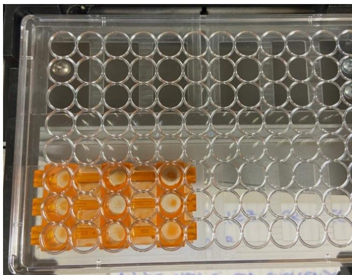
Figure 3.8 Lid and support in PMMA to perform the measurement
