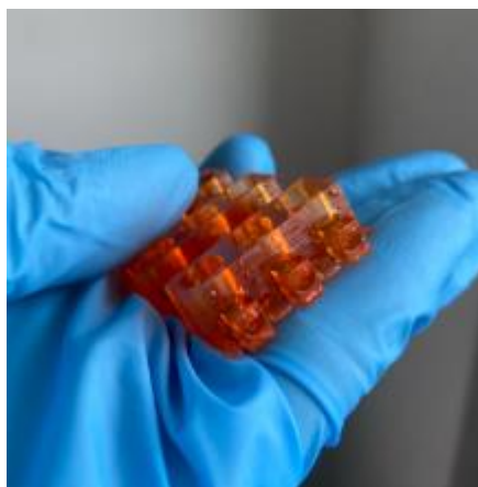
Figure 4.8 Smart plate with final formulation (Disperse Red 1 methacrylate)
