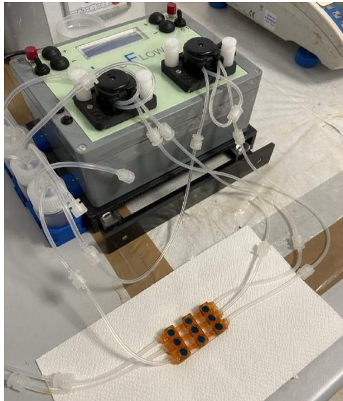
Figure 4.25 Set-up for experimental test on smart plate
