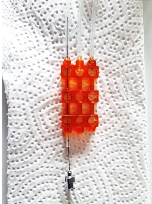
Figure 4.36 Occlusion channels of the smart plate cona go of stainless steel with diameter d=0.7\text{ mm}
