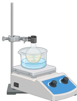
Figure 3.2: Experimental setup used for GelMA synthesis.
