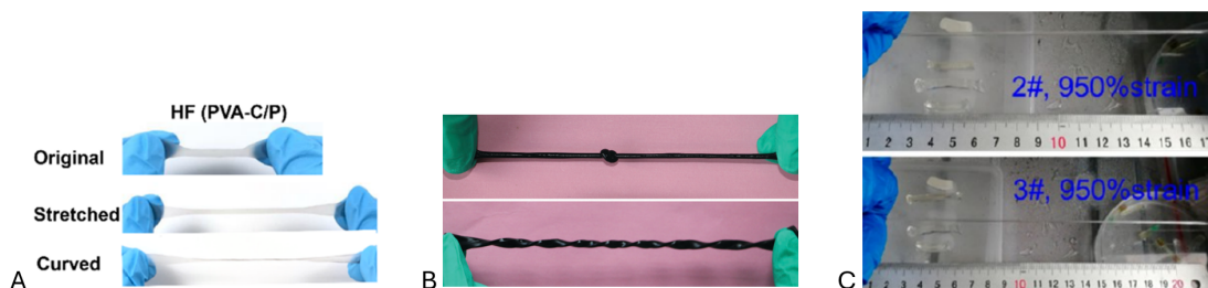
Figure 2.10: Mechanical properties of different hydrogels. A) Hydrogel prepared by Zhang et al. [51], B) Hydrogel prepared by Xia et al. [49], C) Hydrogel prepared by Wu et al. [52].
