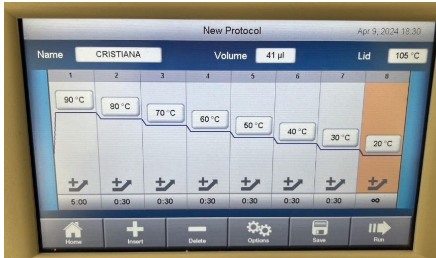
Figure 23 Thermal cycle to hybridize C and C' strands.
