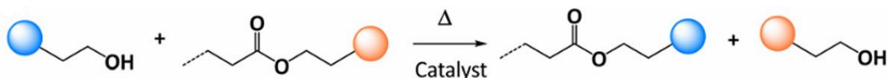
Figure 7: Transesterification reaction between an ester to an alcohol to obtain another ester and another alcohol[3]
