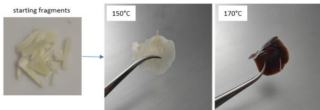
Figure 46: creation of thin films: from starting fragments to films created at 150°C and 170°C
