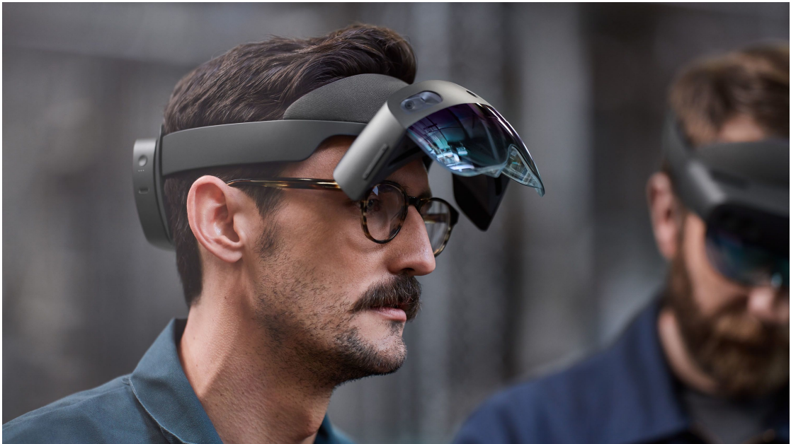
Figure 2.1: HoloLens2 worn by user in flipped up mode
