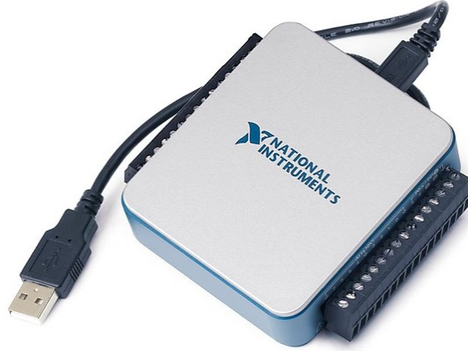
Figure 3.15: National Instruments USB 6001 data acquisition board [5]
