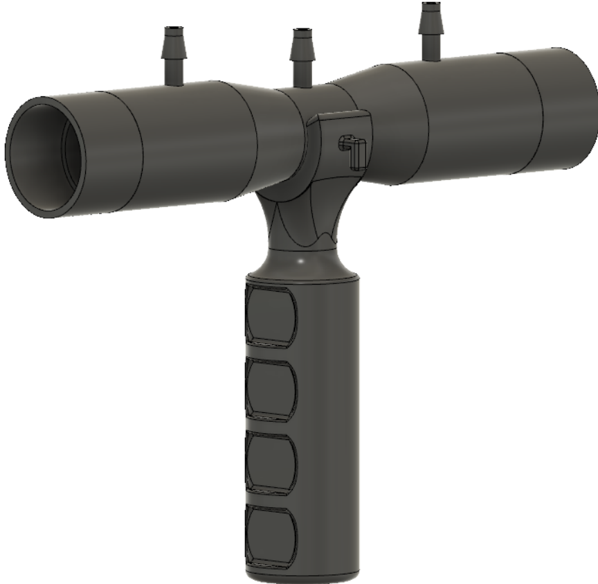
Figure 3.9: 3D representation of the spirometer and handheld grip
