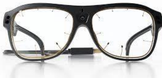
Figura 4.6 Occhiali eye tracking Tobii Pro Glasses 3 ( https://www.tobii.com/products/eye-trackers/wearables/tobii-pro-glasses-3 )
