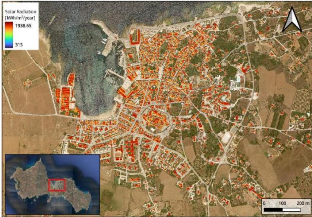
Figure 3 Solar Radiation for rooftop mounted PV
