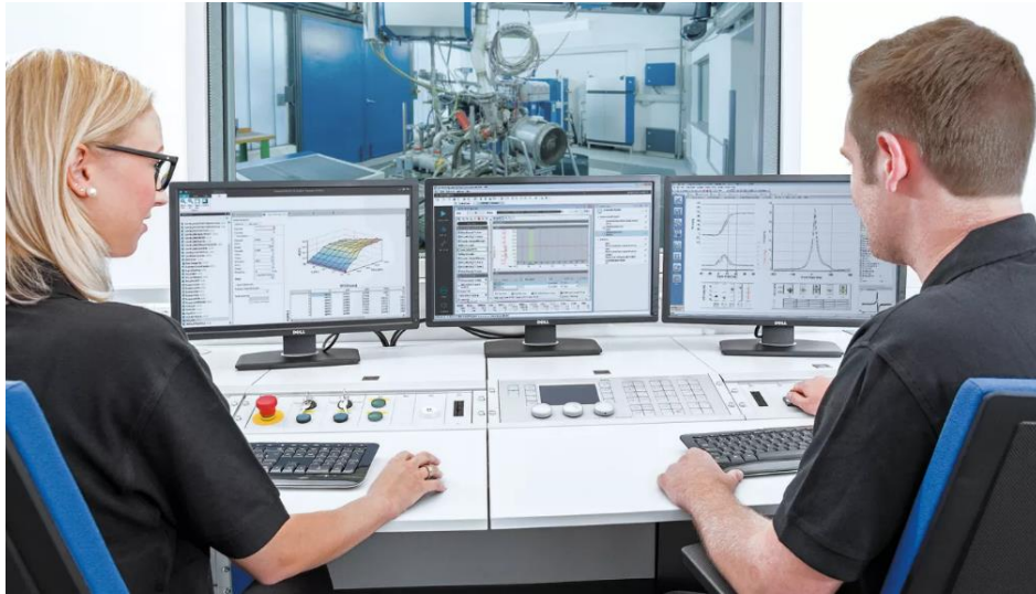
FIGURE 4.3 - DASHBOARD AND CONTROLS OF THE TEST BENCH CELL
