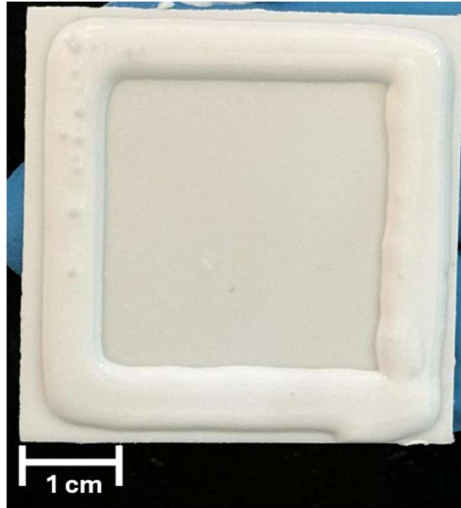
Figure 3.44 Printed shape with the parameters of Table 3.15 on 3YSZ substrate
