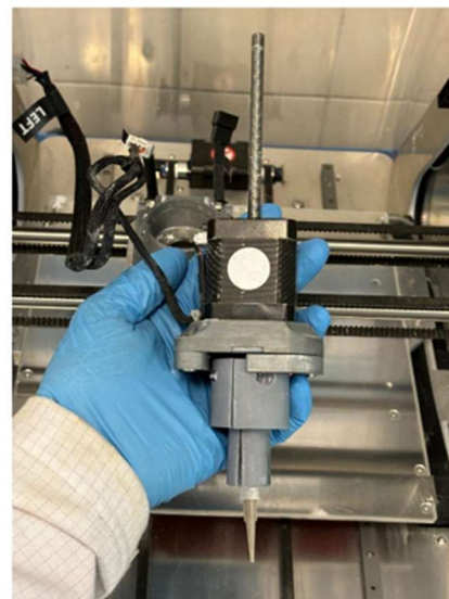
Figure 2.14 a) ZMorphVX 3D printer; b) Thick paste extruder toolhead
