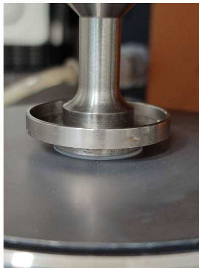
Figure 2.12 Measurement setup of the rotational rheometer head
