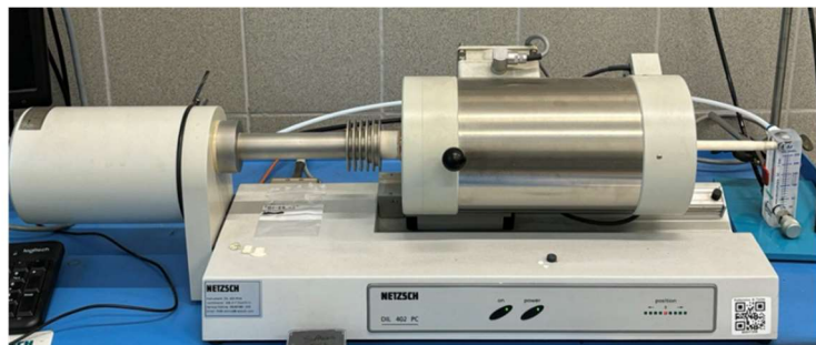
Figure 2.8 Sketch and picture of the dilatometer DIL 402 Expedit Classic [101]
