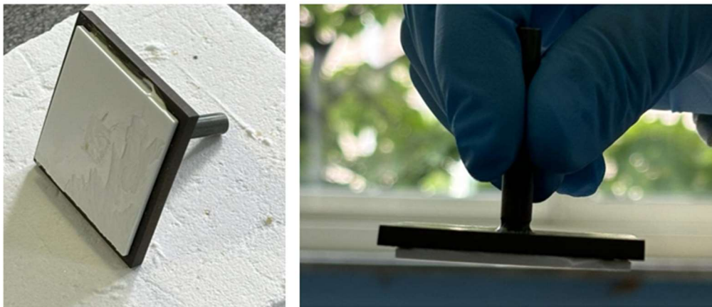
Figure 3.45 Sample for high-pressure tightness test
