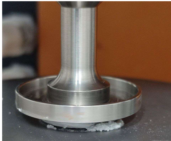
Figure 3.12 Frame of the end of the Flow Sweep Test for MO-SCI 1862 paste, where it is possible to see ink outflow and rapture from the geometry
