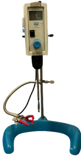
Figure 2.9 Mechanical stirrer for the mixing of the pastes
