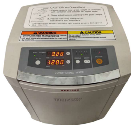
Figure 2.10 Picture of the THINKY ARE-250 planetary mixer
