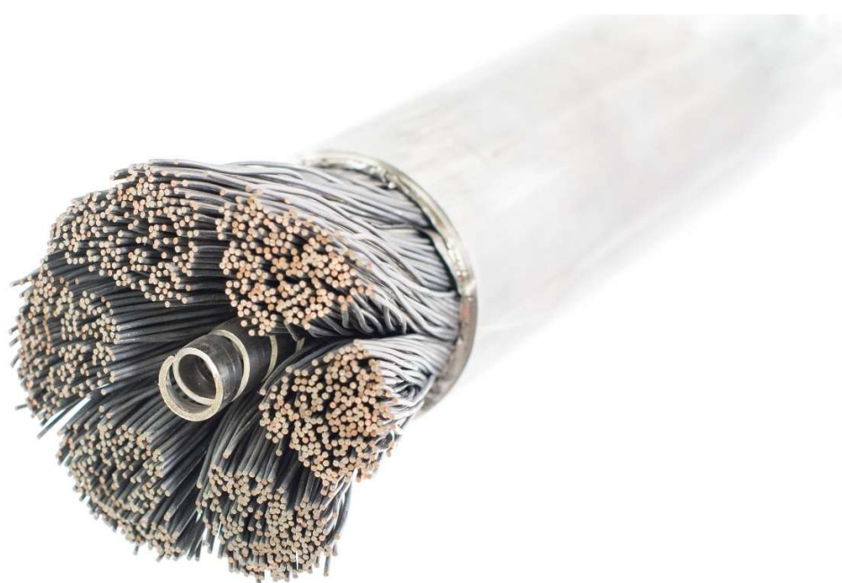
Figure 1.2 – 1: Exposed view of a Nb 3 Sn ITER-like cable for toroidal field coils. Images by Charlie Sanabria. SULTAN-tested cable was provided by courtesy of Pierluigi Bruzzone (Plasma Physics Research Center) with agreement from Fusion for Energy.
