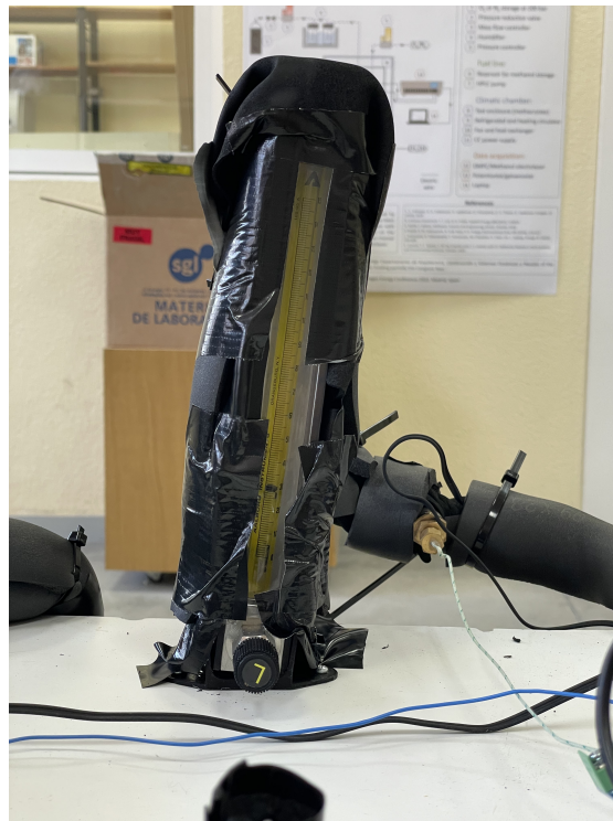
Figure 7.8: Flowmeter with neoprene
