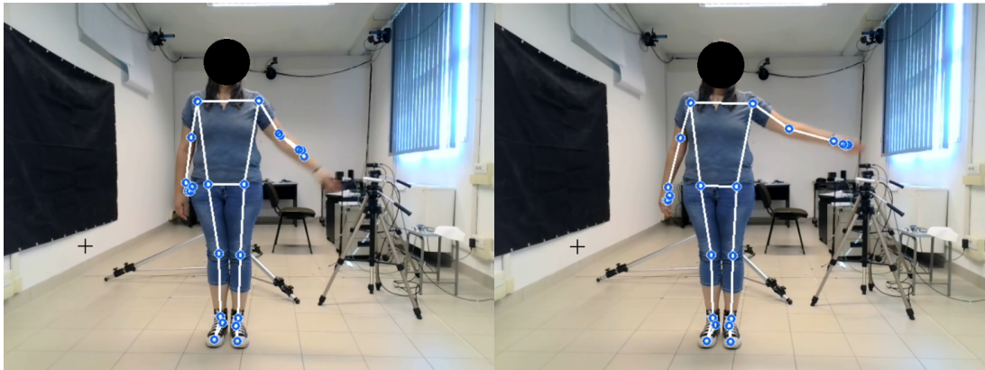
Figure 4.1: Examples of wrong and good pose estimation with good lighting, but complex background (wrong positions for wrist and hand joints)
