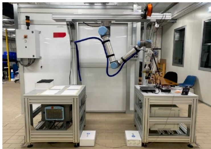
Figure 16: UR10e work cell.
